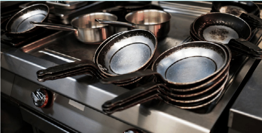
FIGURE 5.26: WARPED AND BURNT PANS ARE EXTREMELY COMMON IN CONVENTIONAL COMMERCIAL KITCHENS
